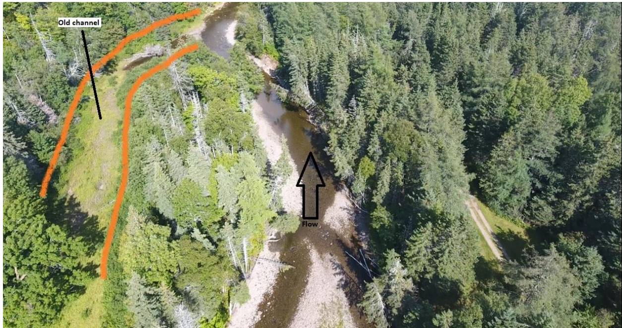
Figure 22: 500 meters Above Moran Road bridge, severe channel migration caused by over-widened channel above.
