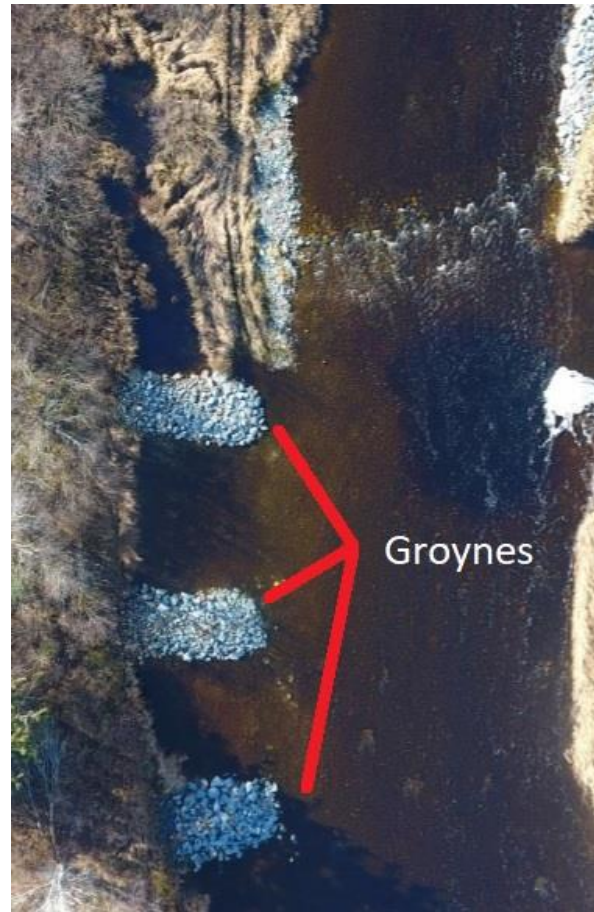
Figure 47: Deflector Design (DFO, 2006)
