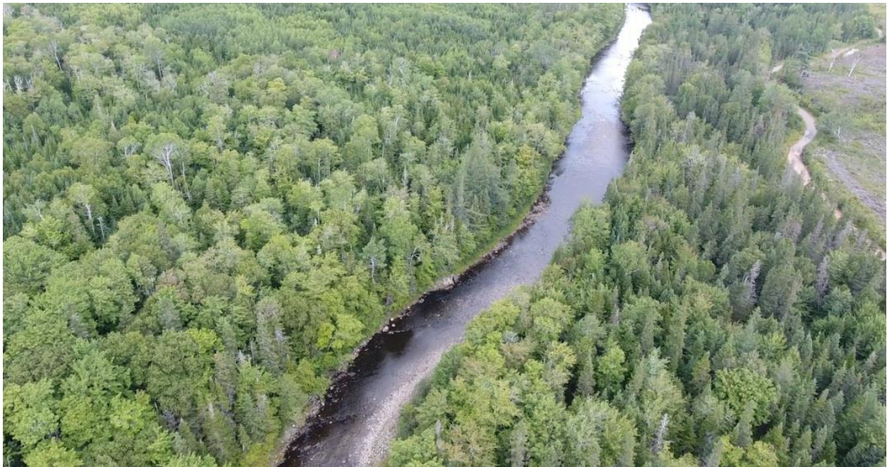
Figure 41: Upper Southwest Mabou (looking downstream) in MacLeod Settlement. Note the channel is over-widened and lacks a meander pattern.
