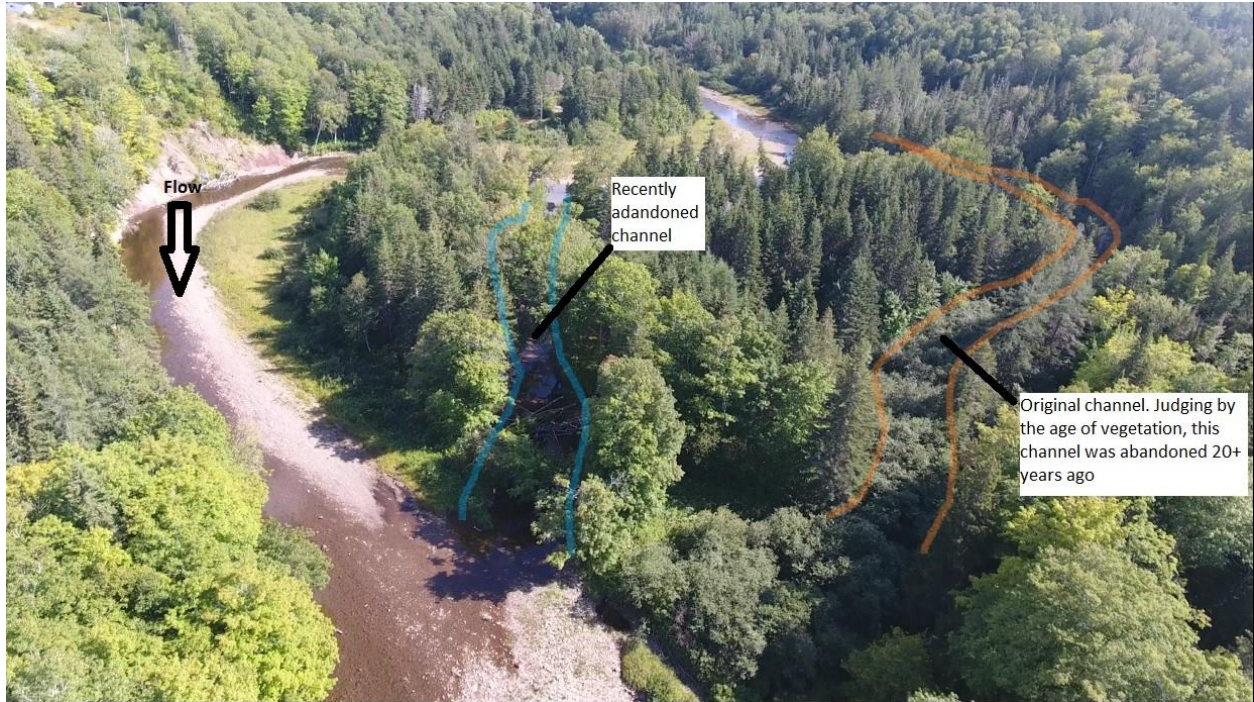
Figure 24: 2.5km above Moran Road bridge. Note - severe channel migration because of incised upstream habitat.
