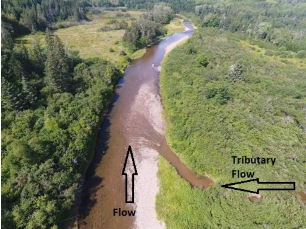
Figure 10: Entrance of small tributary. Over-widened channel limits fish passage from SW Mabou to tributary.
